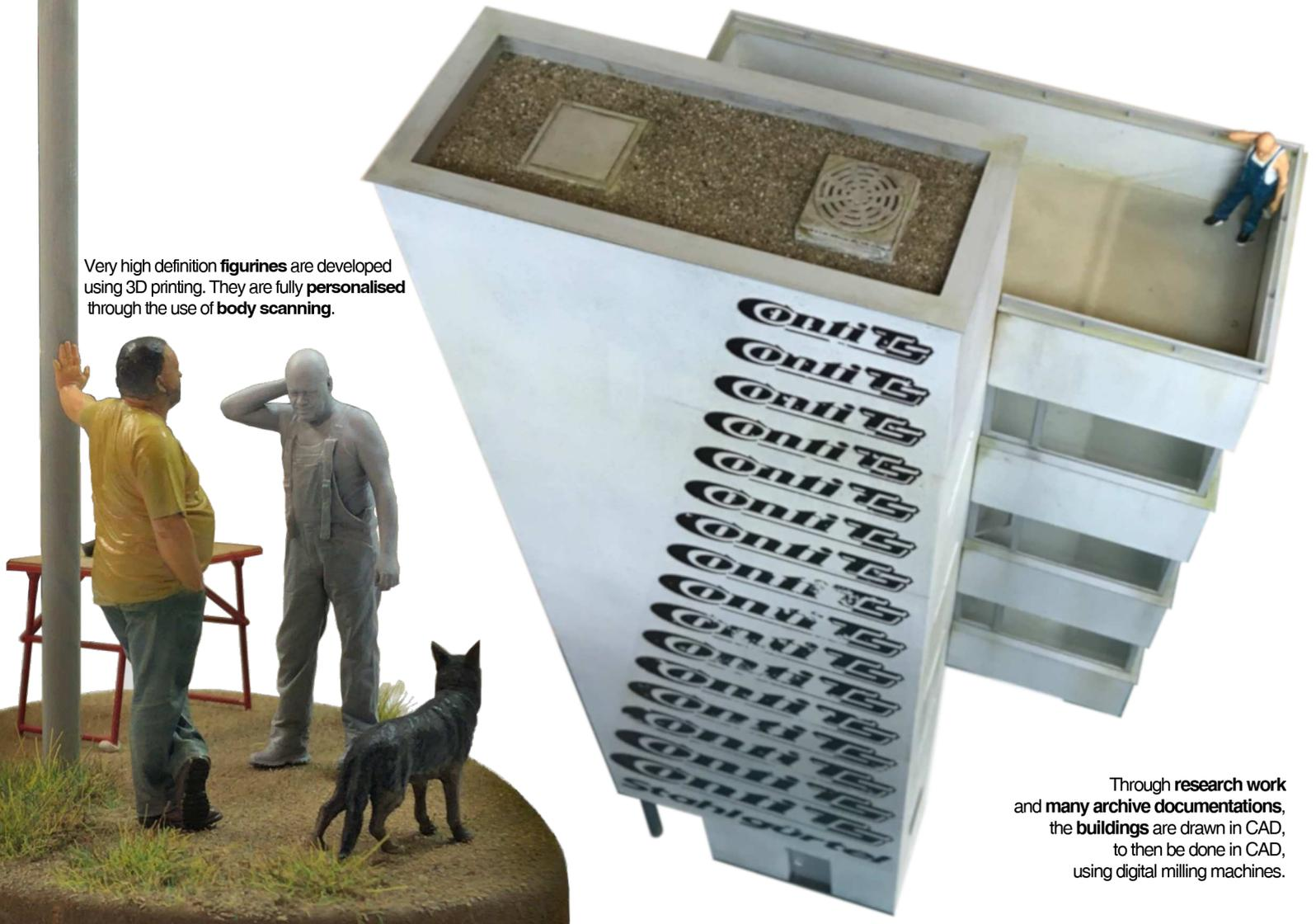
Through **research work** and **many archive documentations**, the **buildings** are drawn in CAD, to then be done in CAD, using digital milling machines.
